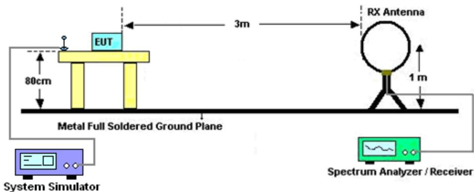
For radiated emissions from 30MHz to 1GHz
