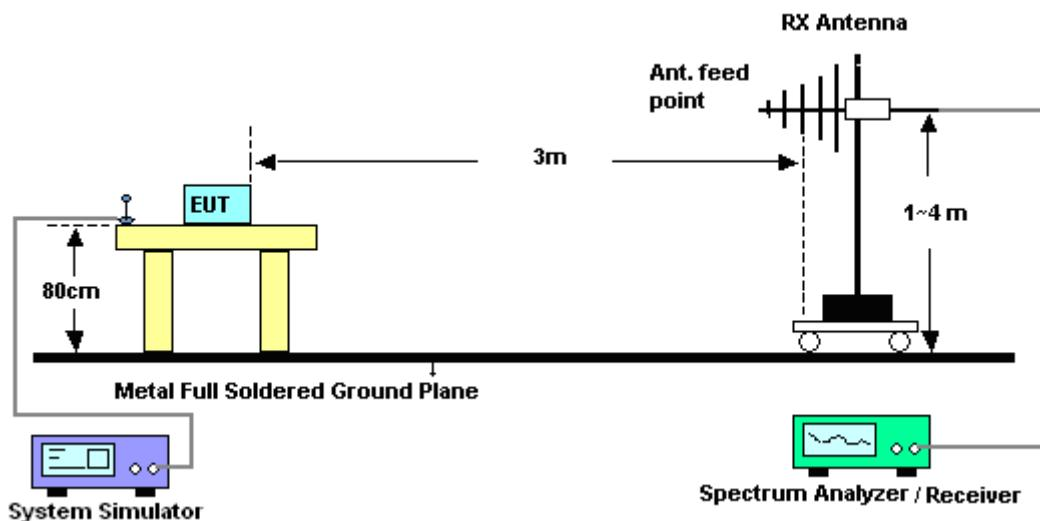
For radiated test above 1GHz
