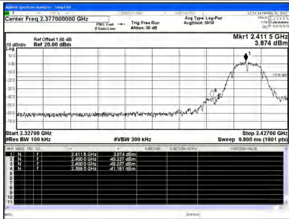
Band Edge NVNT b 2412MHz Ant1 Emission
