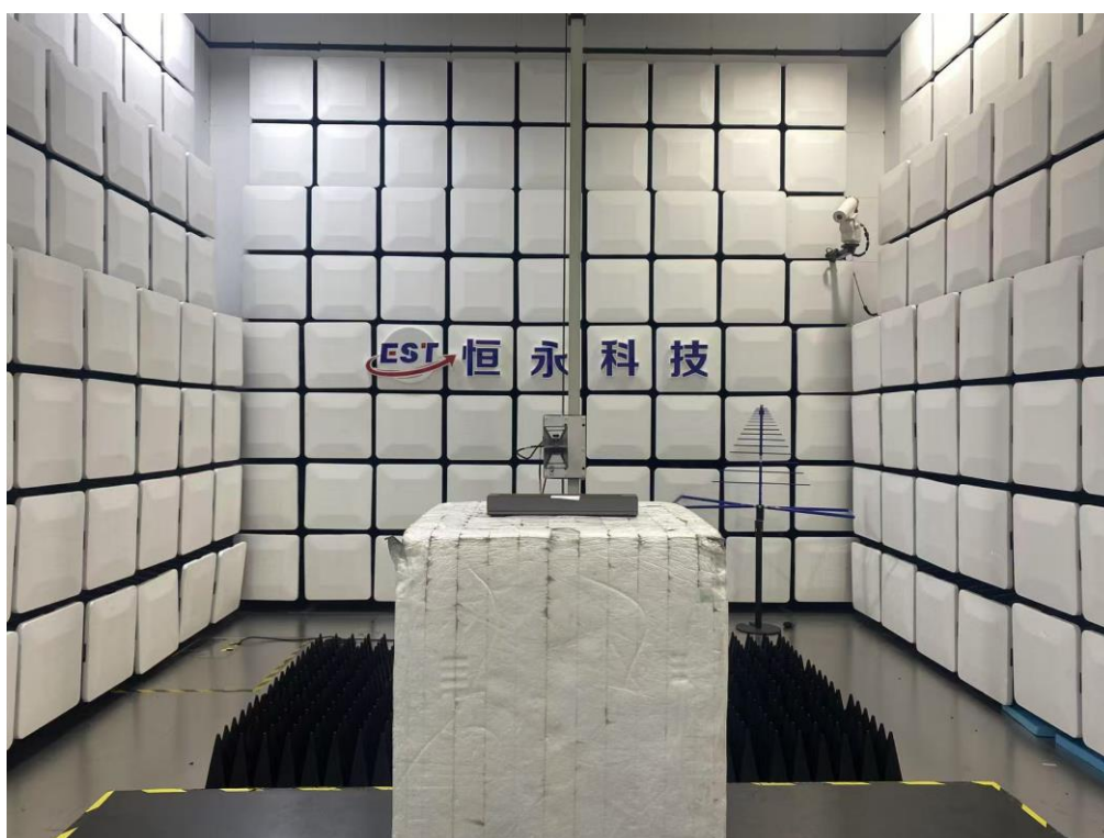
Radiated emission test: Above 1GHz
