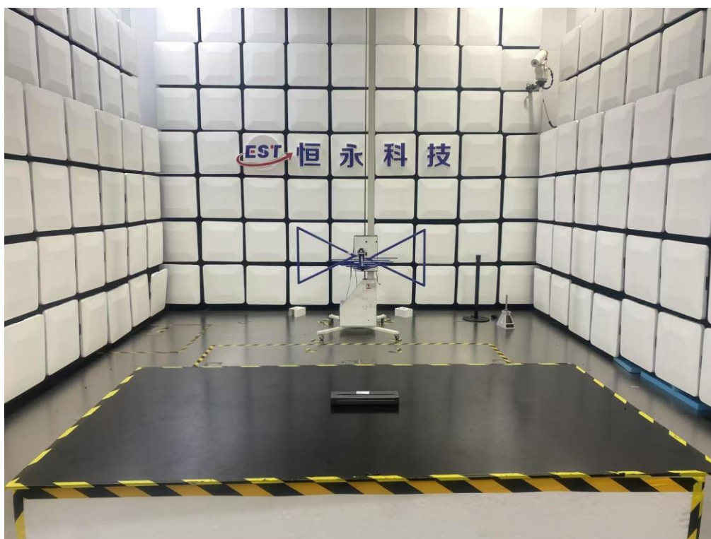
Radiated emission test: Below 1GHz
