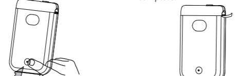
① When installing or replacing the label roll for the first time, the label position identification is required. (Step 01)
