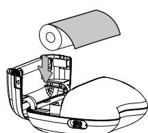
01 Place the paper roll in the printer and pull the paper head out above the paper outlet.
