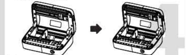
⑧ Pull out the label paper until it is flush with the open button, then close the lid.
