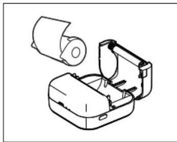
5. Put the printing paper into the paper compartment of the machine and close the top cover
