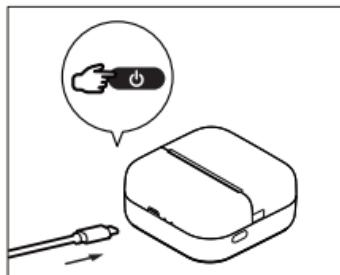
1. Please charge the printer for the first use, and then press and hold the power button for about 3 seconds to turn it on
