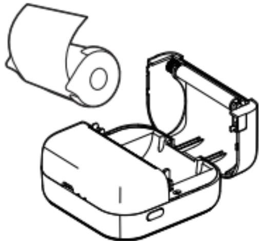
5. Put the printing paper into the paper compartment of the machine and close the top cover
