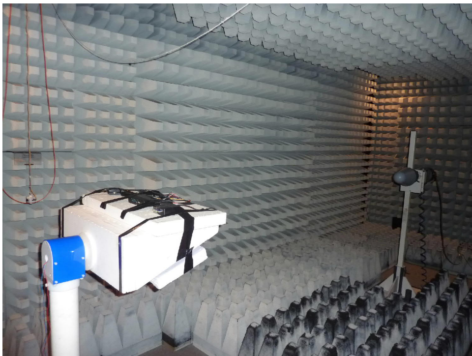
181948_4.JPG : Test setup final measurement from 1 to 14 GHz
