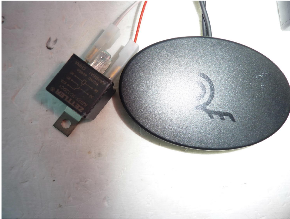
181948_eut5.JPG : Ancillary 12 V DC relais and GNSS antenna
