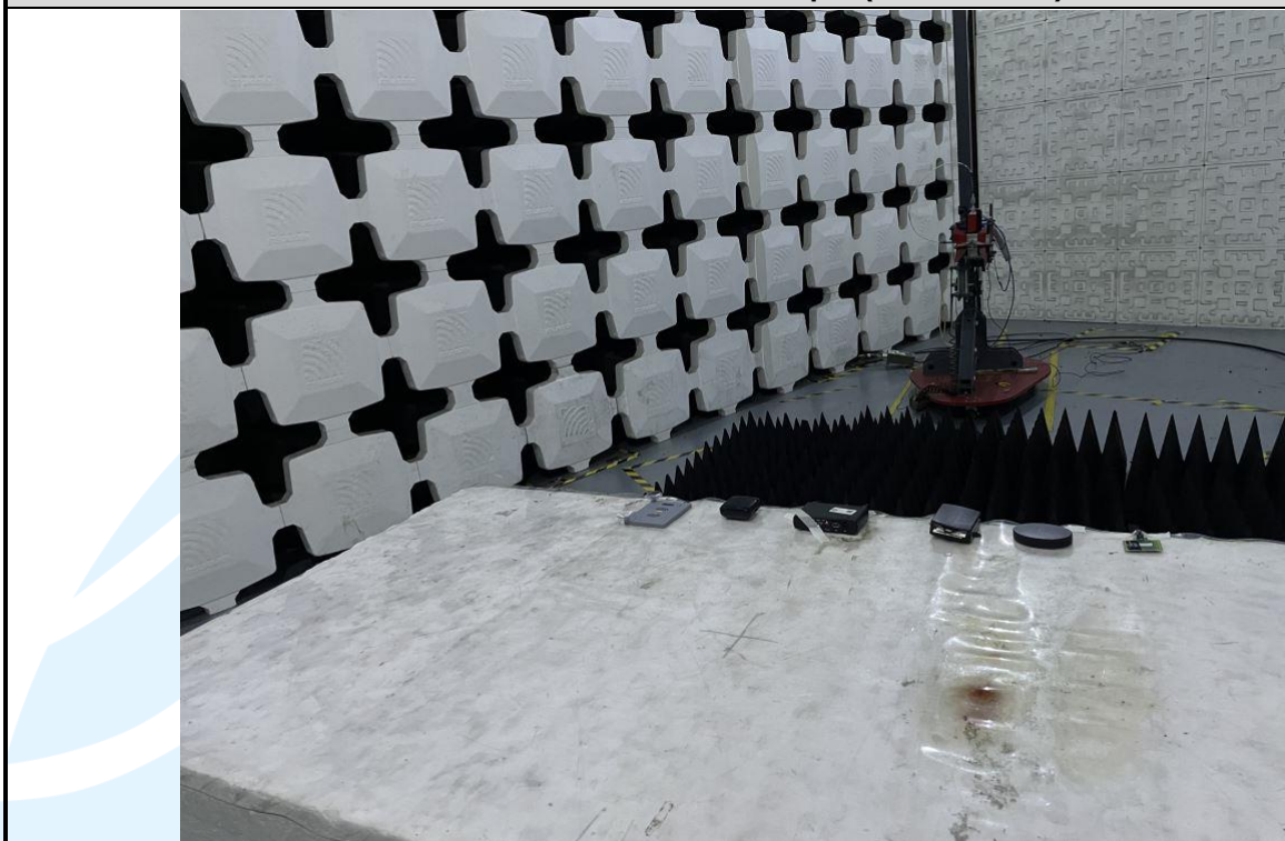
Radiated emission Test Setup-2 (Above 1 GHz)
