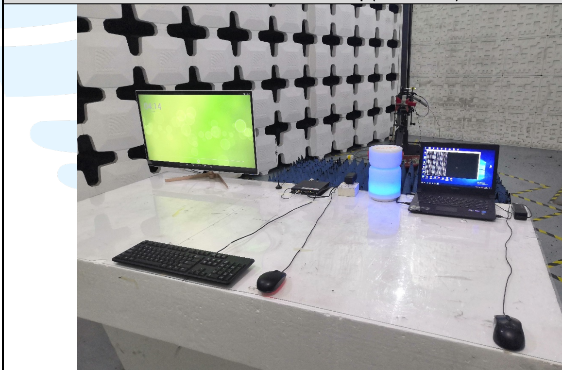
Radiated emission Test Setup (Above 1 GHz)
