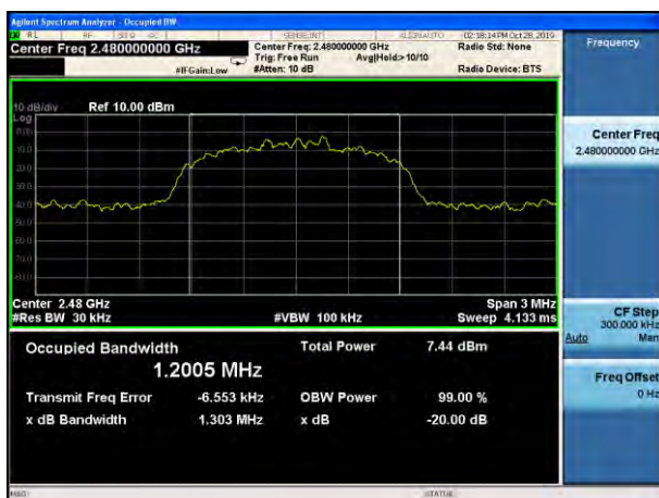
20dB Bandwidth plot on channel 78 (3Mbps)
