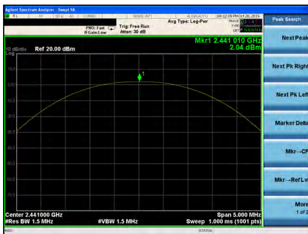
Peak output Power plot on channel 39 (1Mbps)
