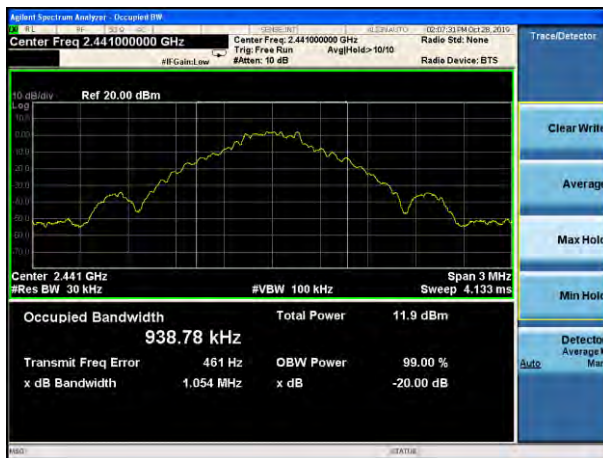
20dB Bandwidth plot on channel 78 (1Mbps)
