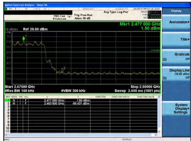
\pi/4 -DQPSK: Band Edge-High Channel
