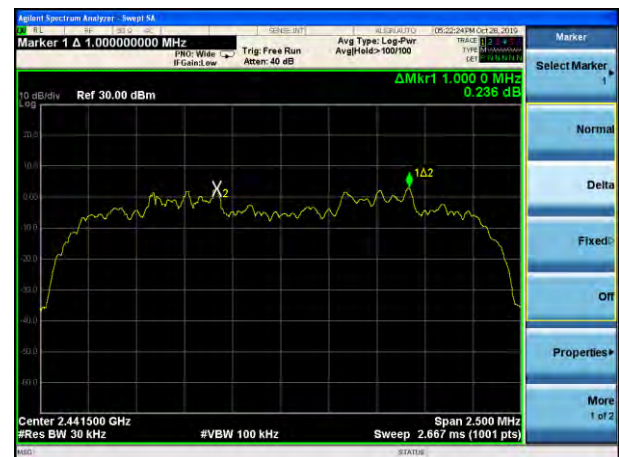
(2Mbps) Channel Separation plot on channel 39-40
