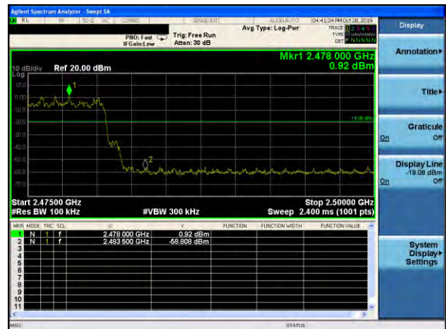
\pi/4 -DQPSK: Band Edge-High Channel
