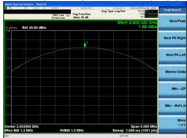
Peak output Power plot on channel 00 (2Mbps)
