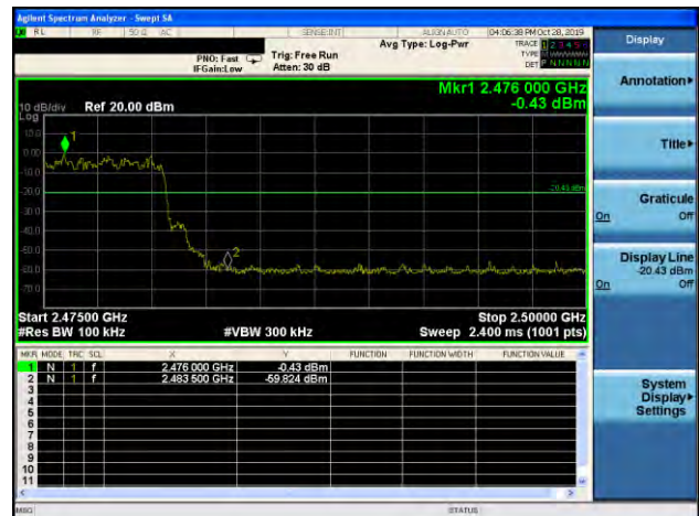
8-DPSK: Band Edge-High Channel (Hopping Mode)
