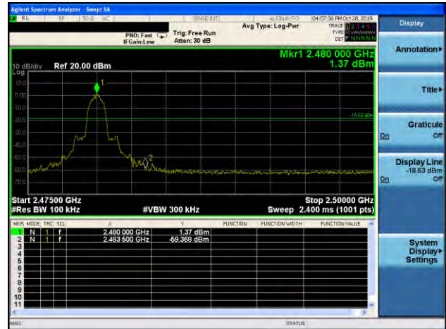
8-DPSK: Band Edge-High Channel
