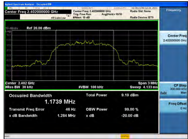
20dB Bandwidth plot on channel 39 (2Mbps)
