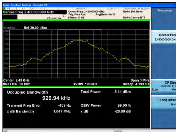
20dB Bandwidth plot on channel 78 (1Mbps)
