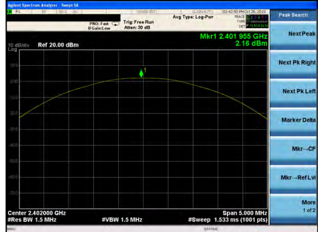
Peak output Power plot on channel 39 (2Mbps)
