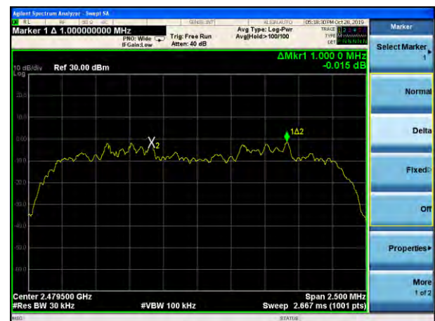
(2Mbps) Channel Separation plot on channel 77-78
