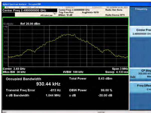
20dB Bandwidth plot on channel 78 (1Mbps)
