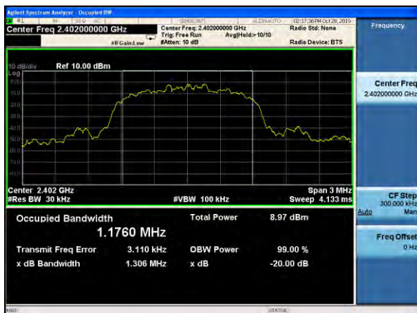
20dB Bandwidth plot on channel 00 (3Mbps)
