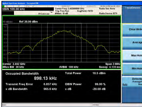
20dB Bandwidth plot on channel 39 (1Mbps)
