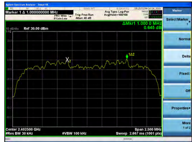
(2Mbps) Channel Separation plot on channel 39-40
