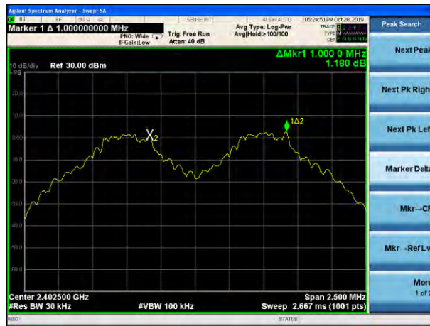
(1Mbps) Channel Separation plot on channel 39-40
