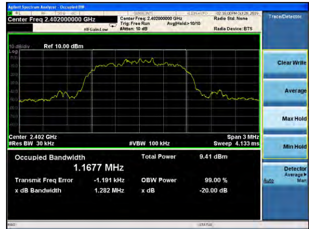
20dB Bandwidth plot on channel 39 (2Mbps)
