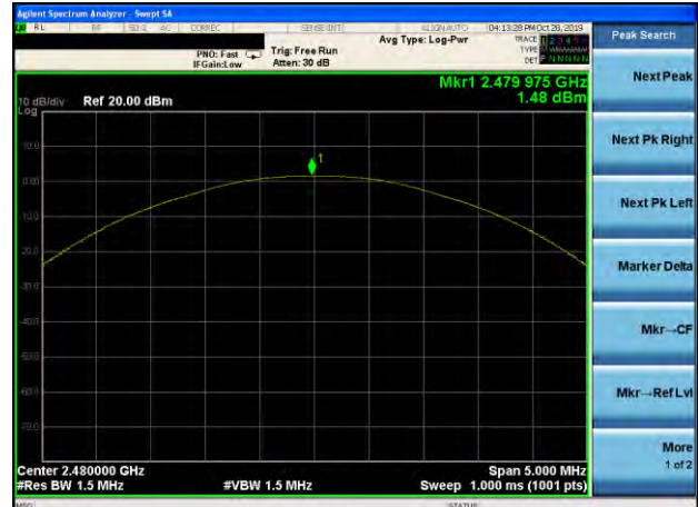
Peak output Power plot on channel 78 (2Mbps)
