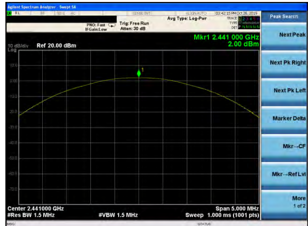
Peak output Power plot on channel 39 (2Mbps)
