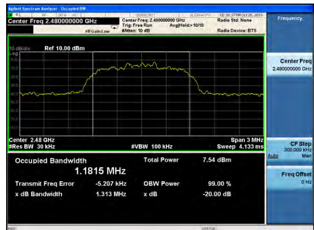
20dB Bandwidth plot on channel 78 (2Mbps)
