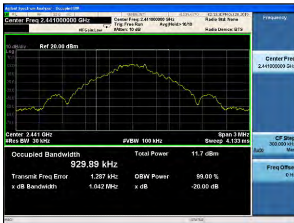
20dB Bandwidth plot on channel 78 (1Mbps)
