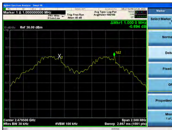
(1Mbps) Channel Separation plot on channel 77-78
