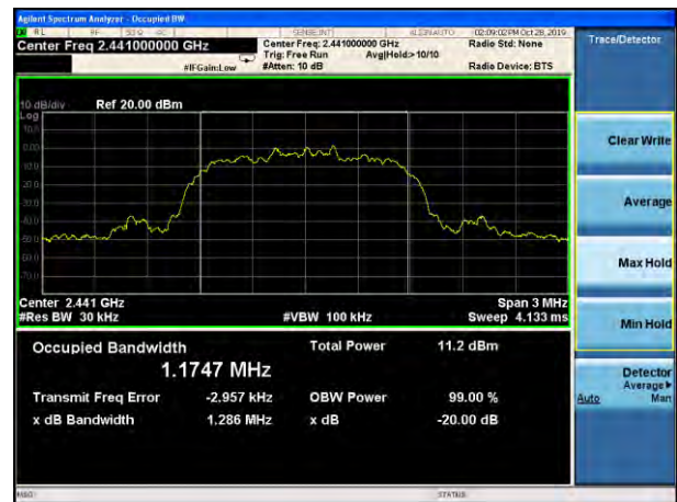
20dB Bandwidth plot on channel 78 (2Mbps)
