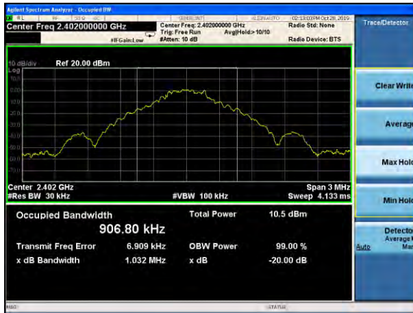
20dB Bandwidth plot on channel 39 (1Mbps)
