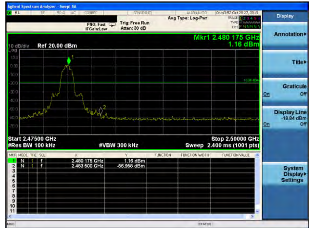
8-DPSK: Band Edge-High Channel
