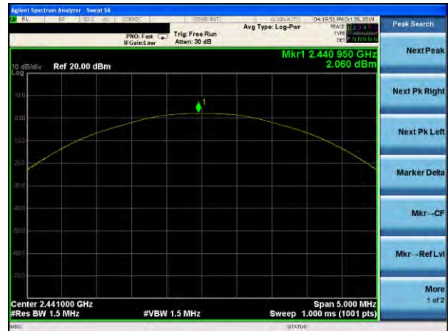
Peak output Power plot on channel 78 (2Mbps)
