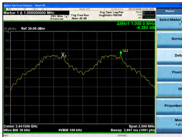
(1Mbps) Channel Separation plot on channel 39-40
