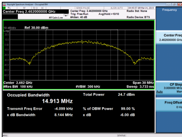
(802.11b) 6dB Bandwidth plot on channel 11
