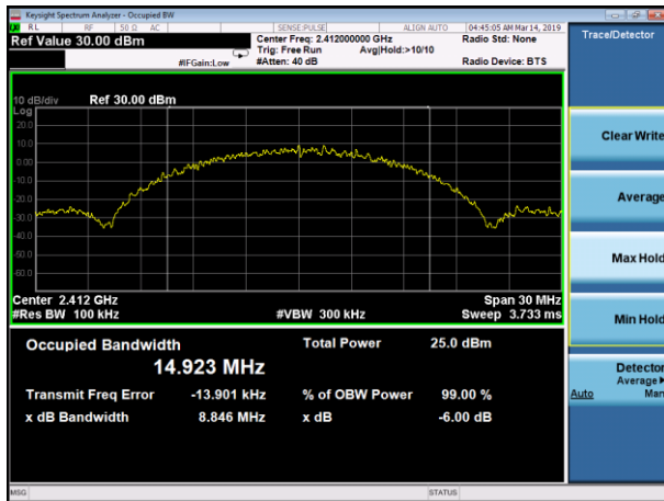
(802.11b) 6dB Bandwidth plot on channel 6
