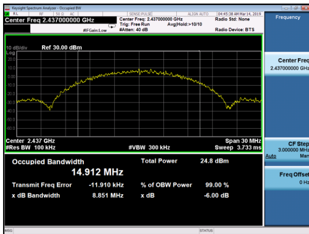
(802.11b) 6dB Bandwidth plot on channel 6
