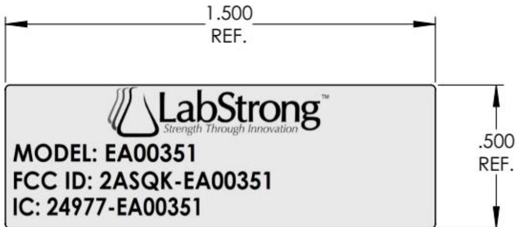
Label printed on **BRADY B-483 THERMAL TRANSFER PRINTABLE LABEL STOCK** and is intended to last the lifetime of the device.
