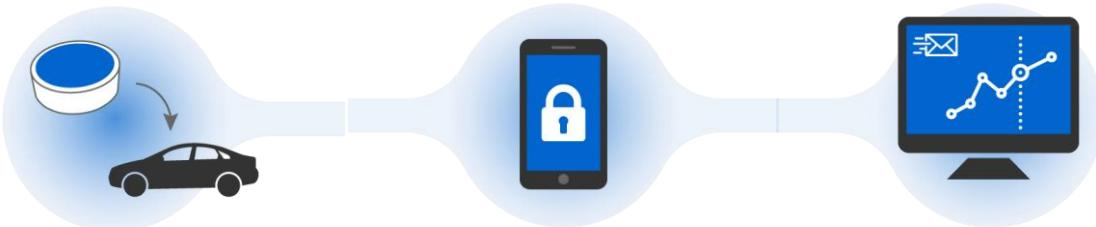
The SafeDrivePod device is placed in the vehicle and detects whether it is moving. The app installed on the phone connects with the pod and closes the screen while driving. The backend server monitors the compliance of the drivers: keep Bluetooth on, keep the app installed, etc.
