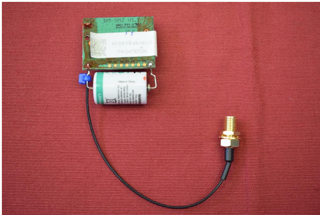
Picture 13: Module with antenna cable – bottom view
