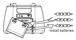
**IMPORTANT:** Be sure that the batteries are installed correctly. Wrong polarity may damage the unit and void the warranty.
