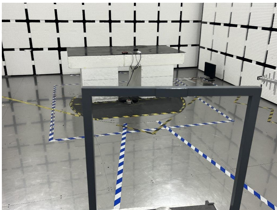
Radiation Emission Test Setup (Below 30MHz)
