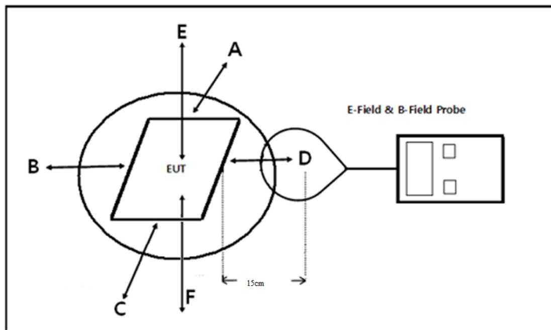
For mobile RF exposure condition, due to installation limitations no tests from the underside of the charging device are required.
