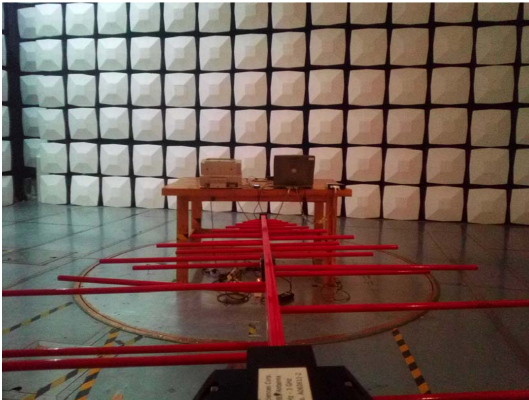
Radiated Emission Below 1GHz Side View
