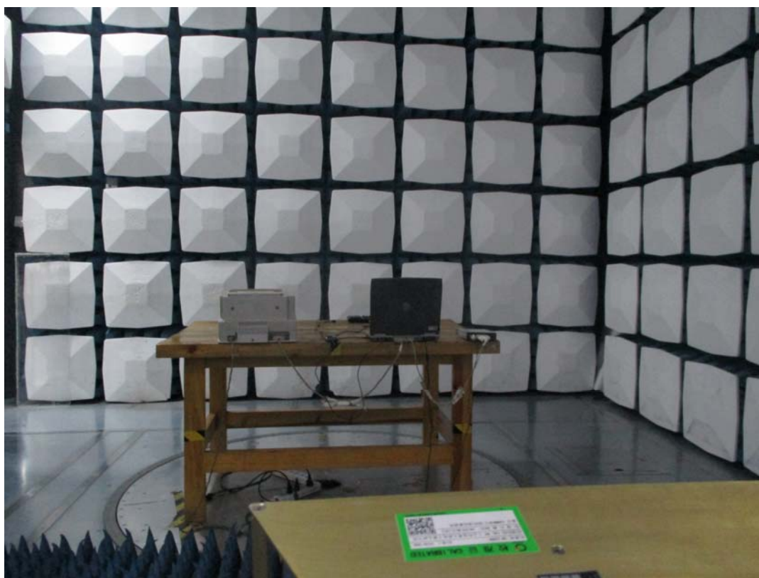
Radiated Emission Above 1GHz Side View
