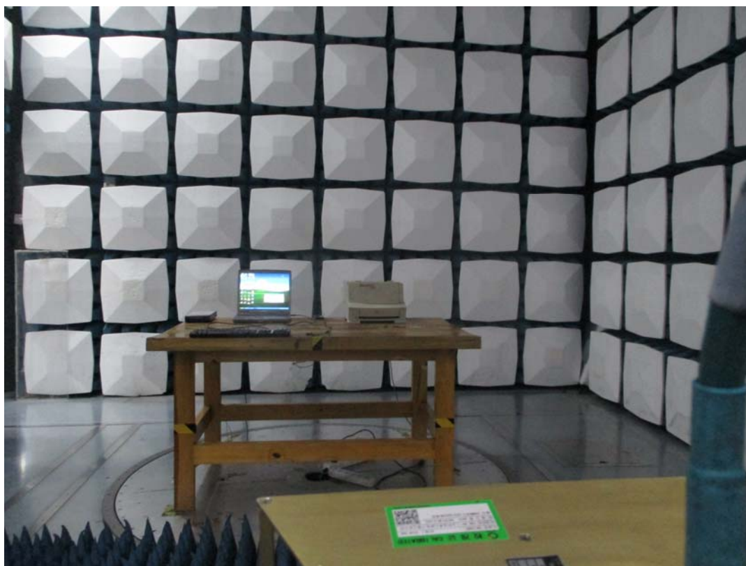
Radiated Emission Above 1GHz Side View
