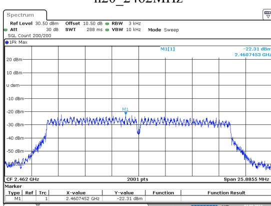
**5.7 100 kHz Bandwidth of Frequency Band Edge**
