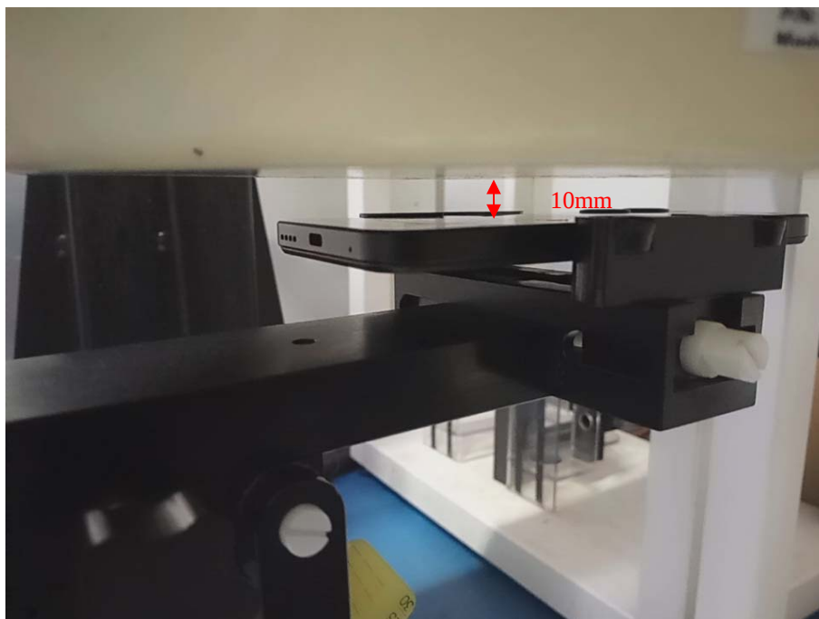
Body(Wron) Back Setup Photo (10mm)
