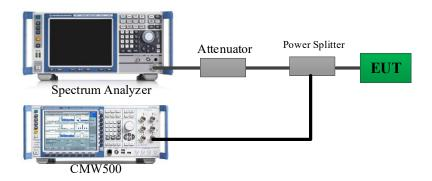
Note: The Insertion loss of the RF cable and Power Splitter was offset into the Reading of Spectrum Analyzer.
