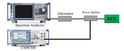
Note: The Insertion loss of the RF cable and Power Splitter was offset into the Reading of Spectrum Analyzer.
