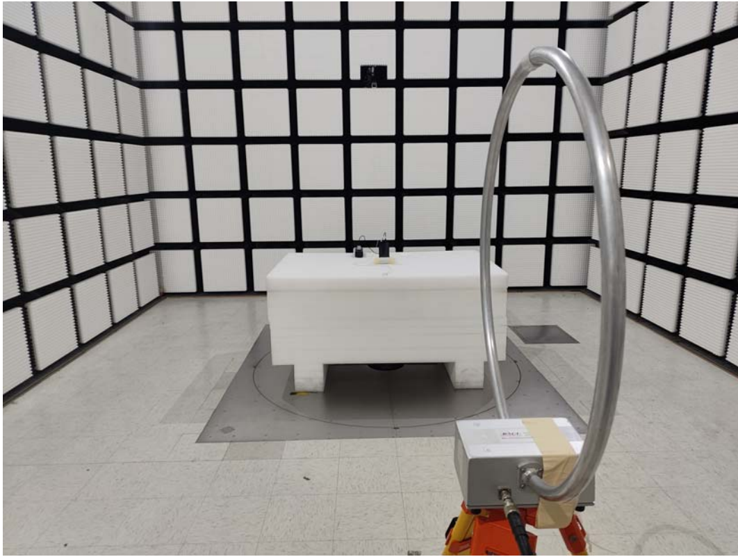
9kHz~30MHz _ Radiated Emission View - Ground-parallel Adapter2
