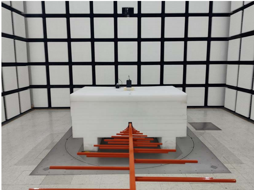
30MHz~1GHz _ Radiated Emission View-Adapter2
