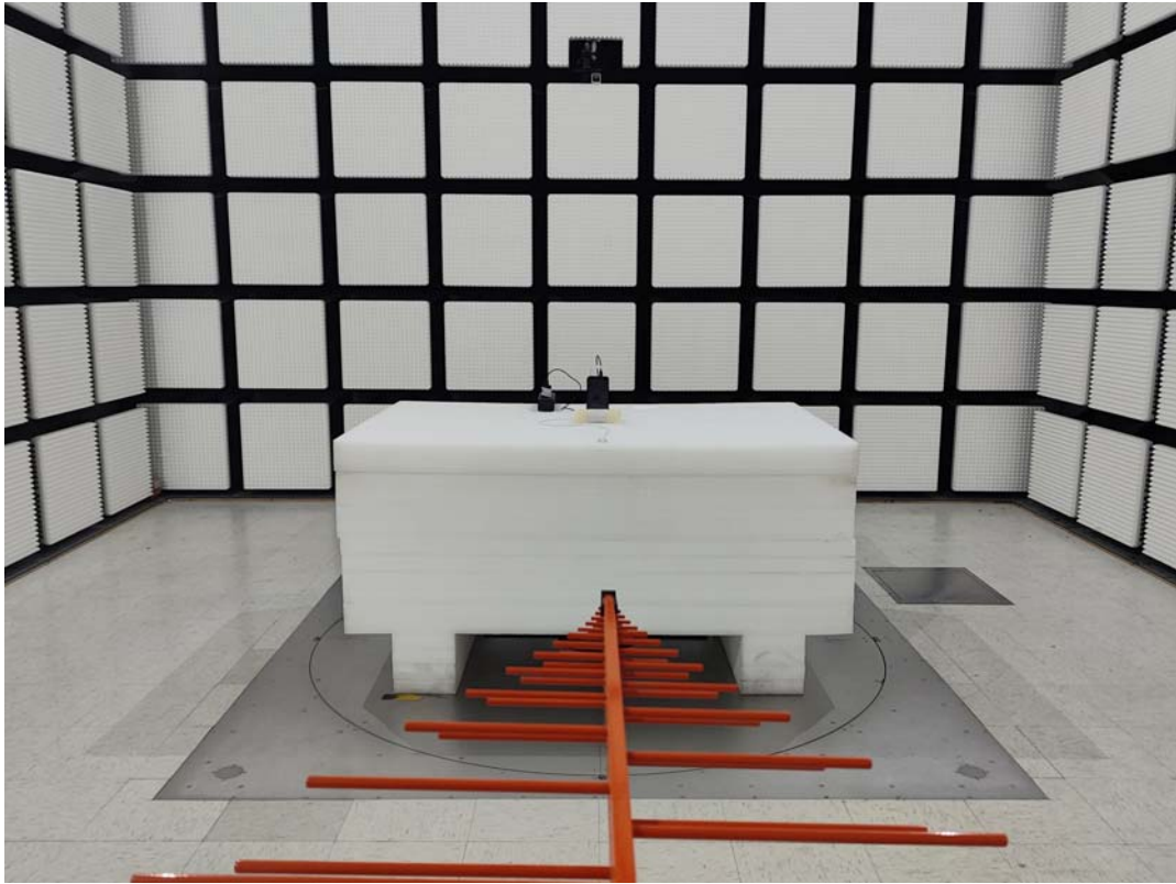
30MHz~1GHz _ Radiated Emission View-Adapter2
