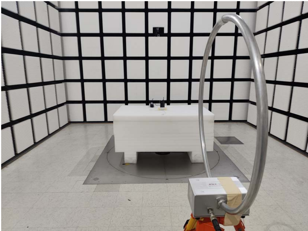
9kHz~30MHz _ Radiated Emission View - Perpendicular_Adapter 1
