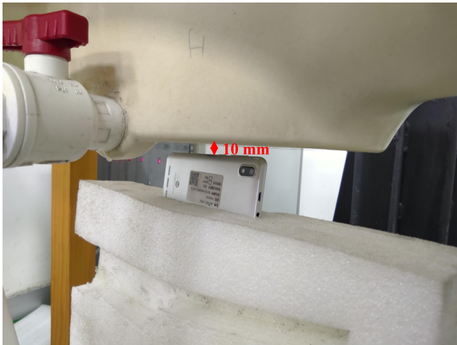
Body Right Setup Photo (10mm)
