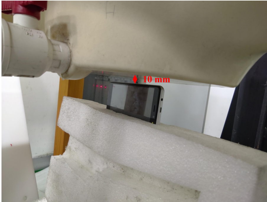
Body Left Setup Photo (10mm)
