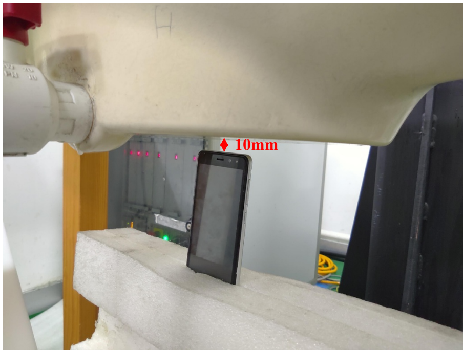
Body Top Setup Photo (10mm)
