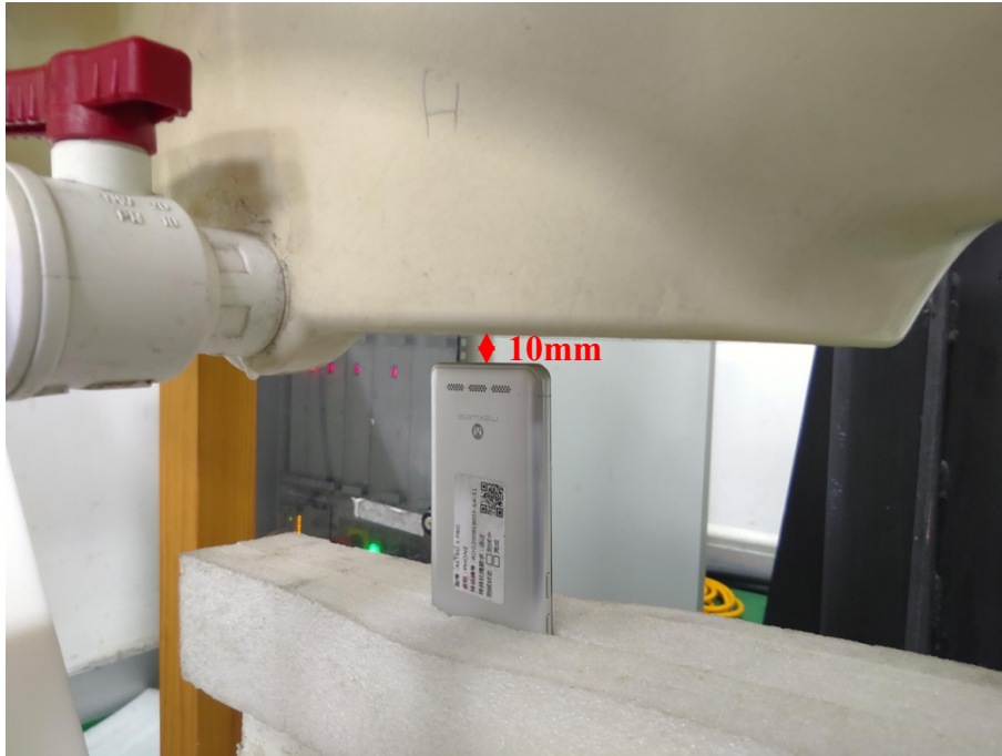
Body Bottom Setup Photo (10mm)
