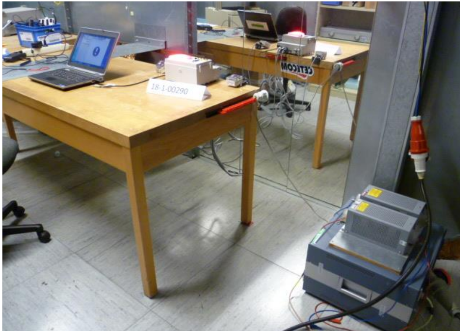
Photograph 5: EUT Setup Conducted emissions on AC-Power lines
