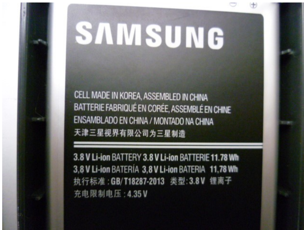
Figure 5: EUT 3.8V Li-ion battery
