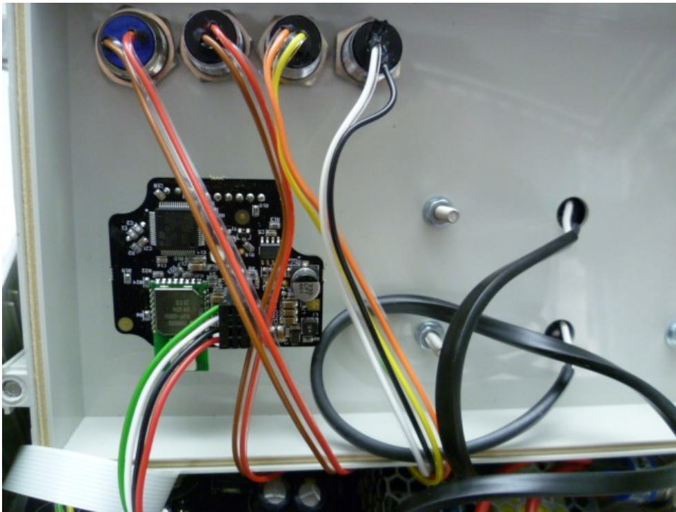
Figure 12: EUT inside view UWB module
