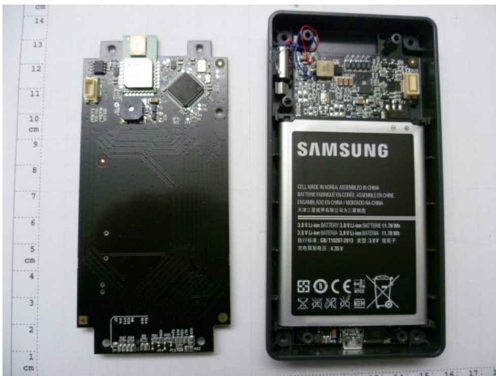
Figure 4: EUT A 3.8V Li-ion battery
