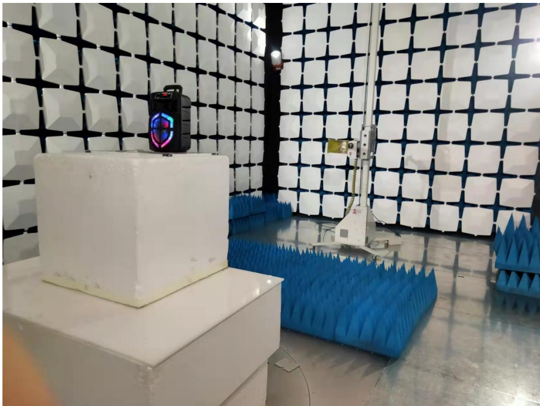
Above 1GHz for radiated emission test setup
