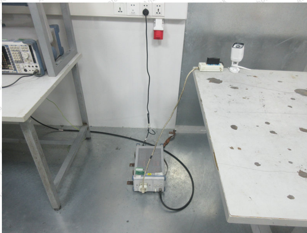
Photo of Power Line Conducted Emission Test
