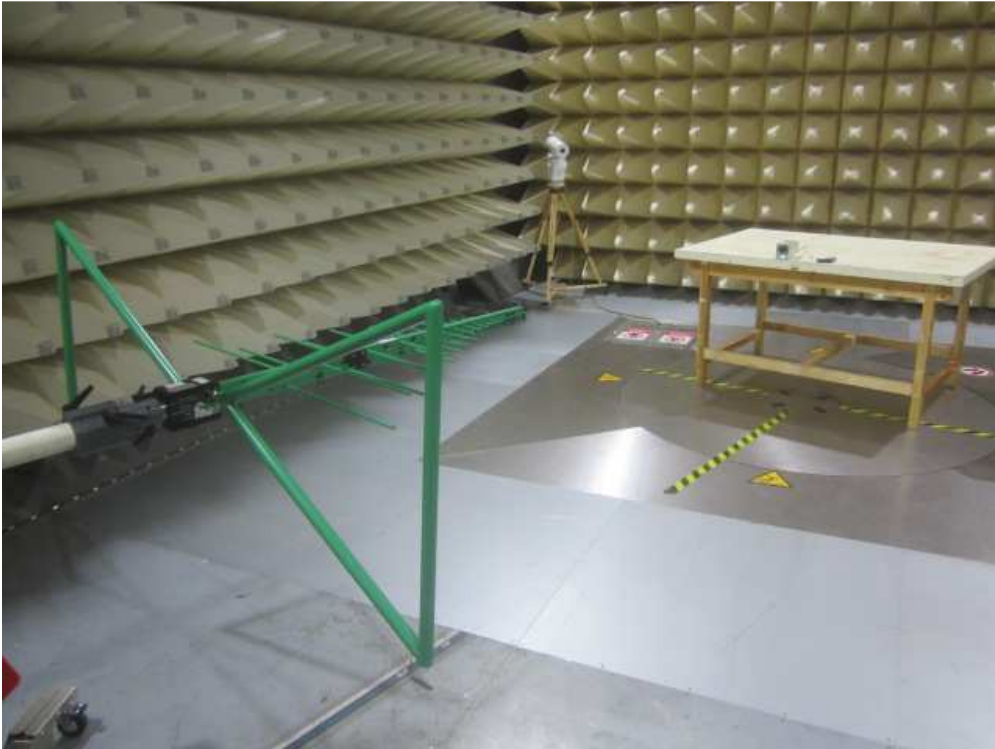
Photograph 1: Set-up for measurement of radiated emission
