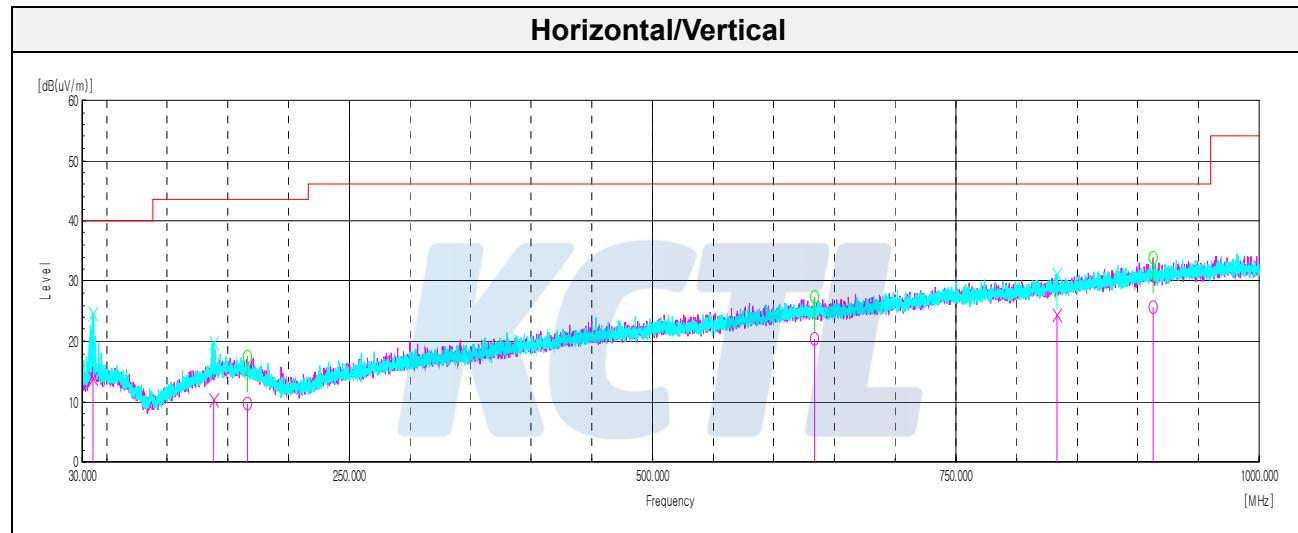
**Test results (Above 1 000 MHz)****802.11n HT20 UNII-1****Lowest Channel (5 180 MHz)**
