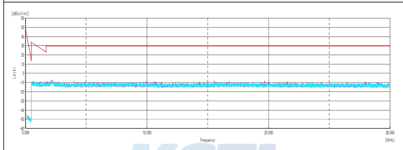
**Test results (Below 1 000 MHz) – Worst case: 802.11n HT20\_UNII-1 Highest frequency**
