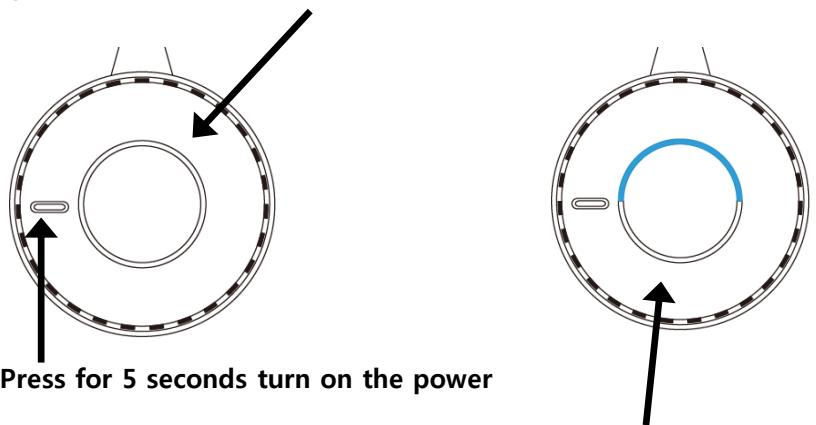
④ Press for 5 seconds turn on the power
