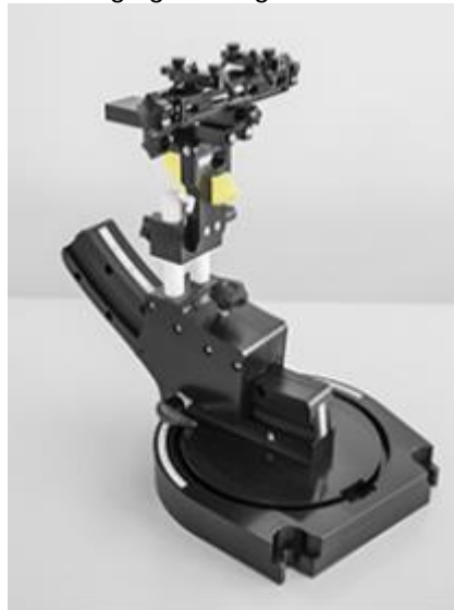
Device holder supplied by SPEAG
