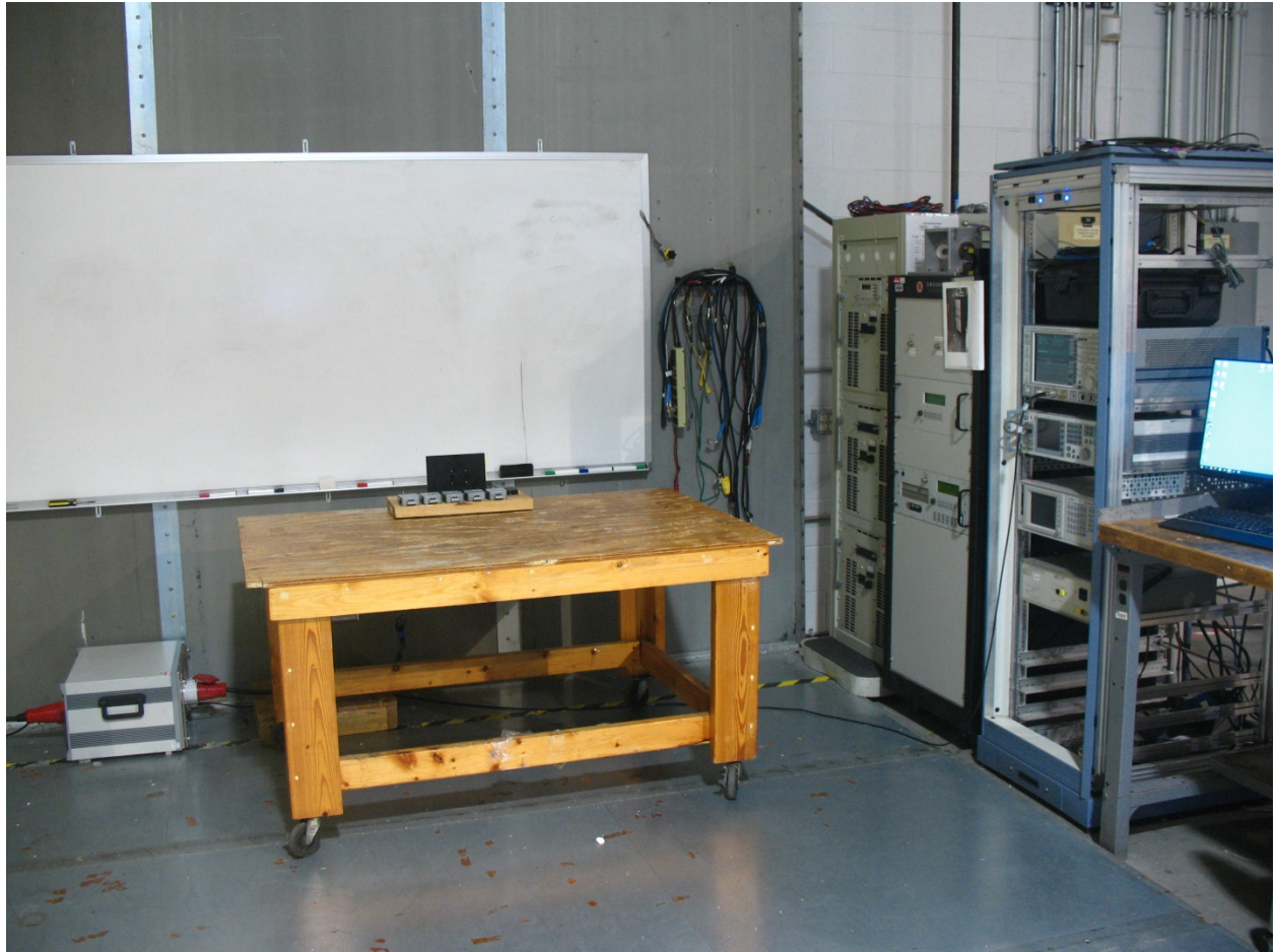
Conducted emissions, 150kHz – 30MHz
