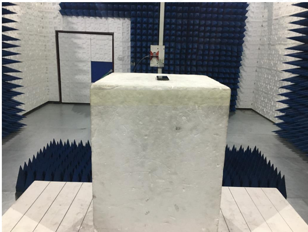
RADIATED EMISSION TEST SETUP ABOVE 1GHZ
