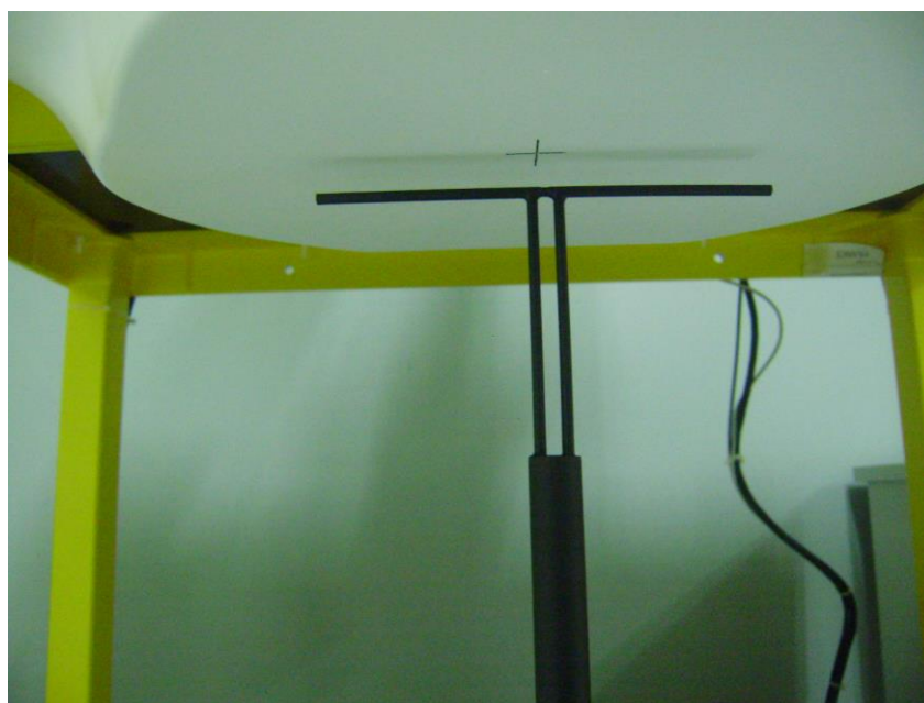
Setup Photo of Dipole Antenna
