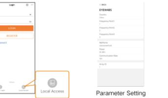
**Step 1:** Open iSolarCloud App, click **Local Access** at the bottom of the login interface, and scan the QR code on the connected inverter to go to the setting interface.
