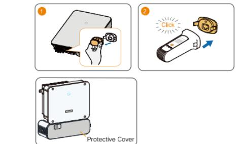
Note: If a protective cover is installed at the inverter bottom, it may cause wireless communication signals to attenuate, thus shortening the communication distance of the communication module.
