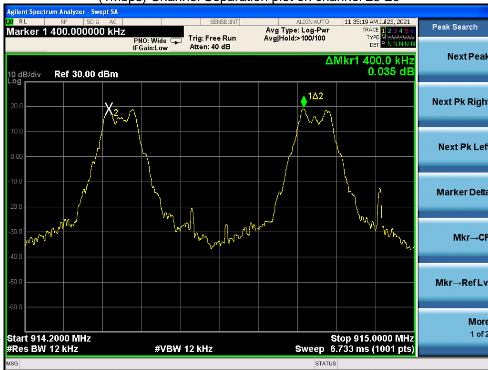
(1Mbps) Channel Separation plot on channel 50-51
