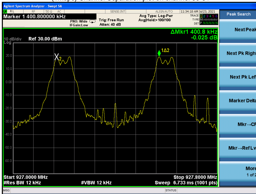
(1Mbps) Channel Separation plot on channel 50-51
