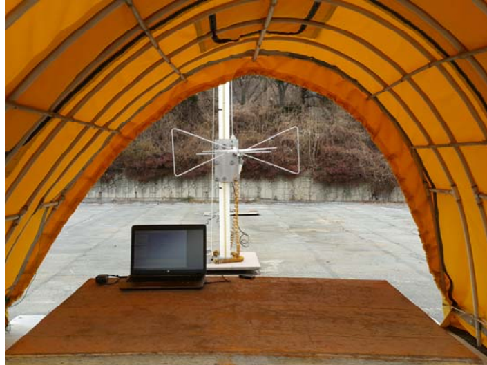
Photograph 2 : Setup for radiated Emissions (above 1 GHz)
