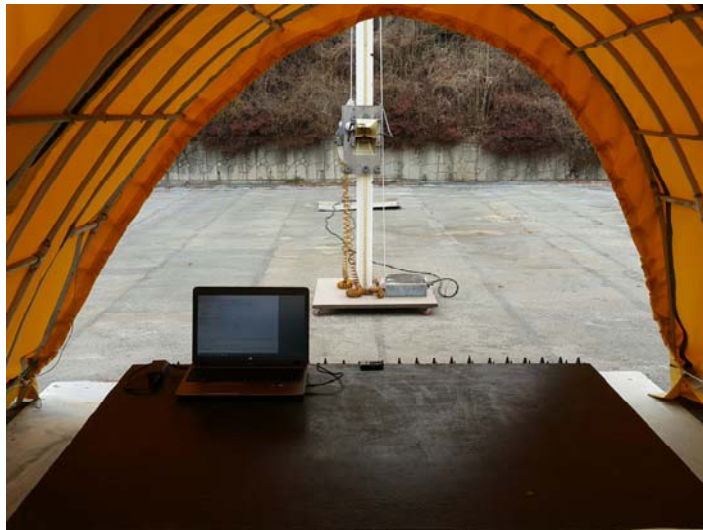
Photograph 2 : Setup for radiated Emissions (above 1 GHz)
