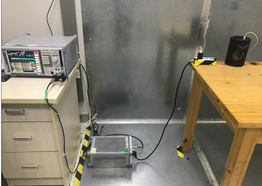
Radiated Spurious Emissions From 30MHz-1000MHz
