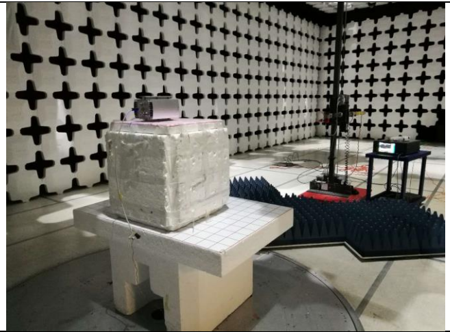
Radiated Emissions above 1GHz Rear View
