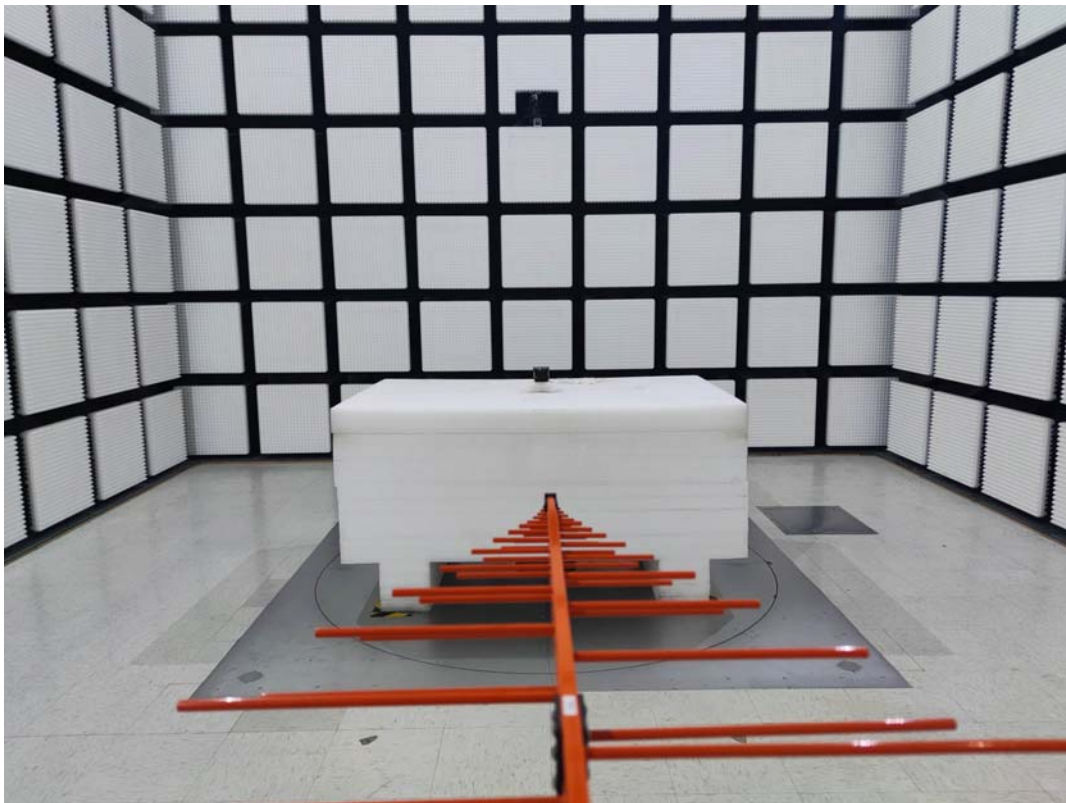
Radiated Emission 30M-1GHz View
