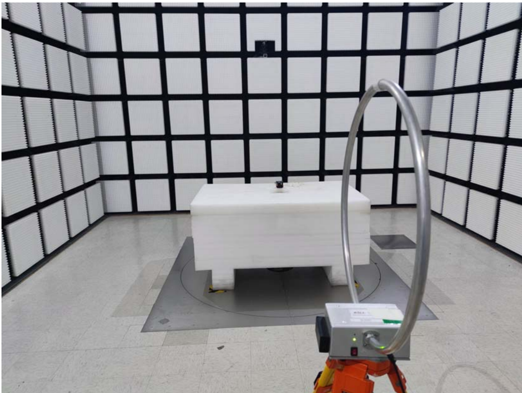
Radiated Emission 9k-30MHz Perpendicular View
