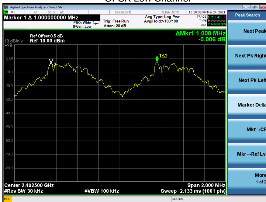
Test plots GFSK Low Channel
