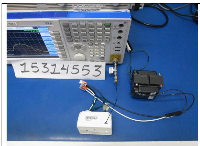
RF ANTENNA PORT CONDUCTED
