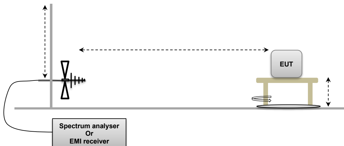
Test setup of Unwanted Emissions in Restricted Frequency Bands
