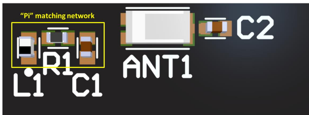
WLA.01 antenna mounted on a PCB, showing “Pi” matching network.
