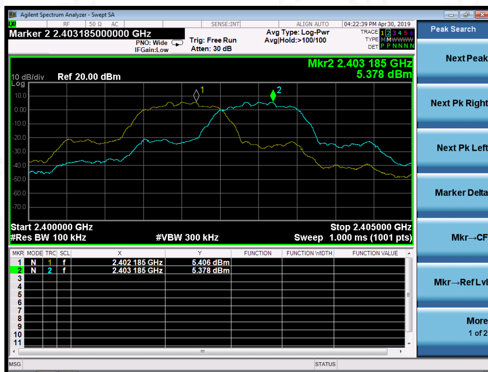
TEST PLOT FOR FREQUENCY SEPARATION
